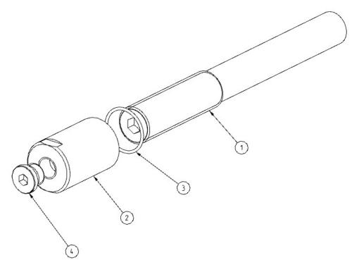
Fig. 9 – Stop protection assembly for cylinder
