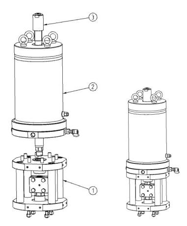
Fig. 1: Main parts for SC/VHS actuator series
