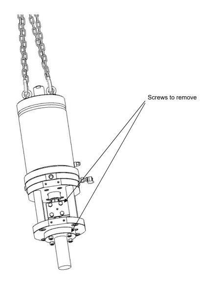
Fig. 4 – Disassembling of the actuator
