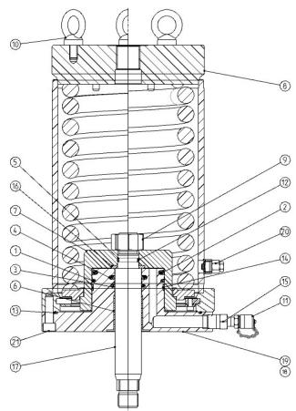
Fig. 8 – Single acting hydraulic cylinder
